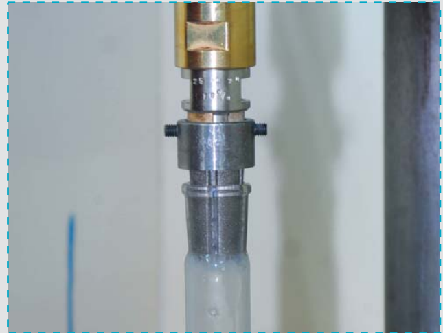
Grinding process of ground joints by diamond reamers.
