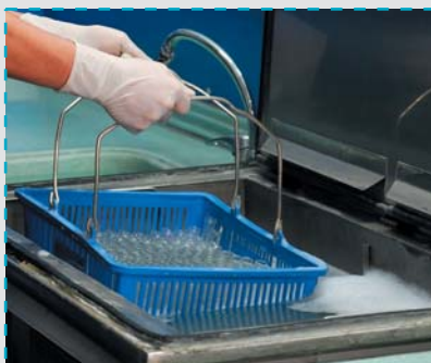
Modern ultrasonic cleaning machines are used to remove all the remaining particles
