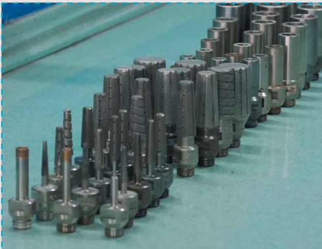
At grinding, only diamond tools are used to yield the perfect results.
